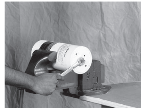
4. Remove the valve adapter and the crush washer from the gas end cap.
