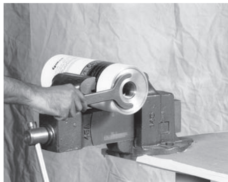
6. Remove the fluid end cap with the end cap wrench.
