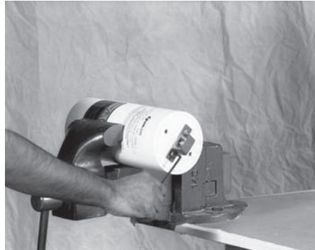
1. Remove valve guard from the accumulator.
