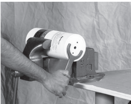
5. Remove the gas end cap with the end cap wrench.
