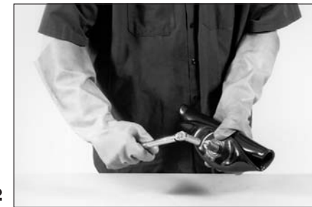
2 Install the valve adapter; tighten to 90 inch-pounds of torque.
