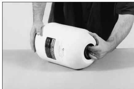
5 Disassembly Remove the jamnut (attached to the valve stem), using a socket wrench, to free the bladder from the accumulator.
