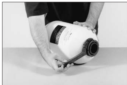
3 Discharge any pressure in the accumulator using the OilAir Hydraulics charging and gauging assembly, OAH Part number TCG-3000 (or CG-5000 for 5 kpsi models).
