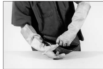
1 Squeeze the bladder to discharge gas from it by rolling it up from the bottom.
