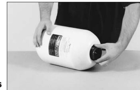
3 Lubricate the accumulator shell and the bladder with system fluid or similar product, then insert the bladder into the shell. Rotate the shell around its axis several times to lubricate the bladder uniformly. ALWAYS WEAR GLOVES! *
