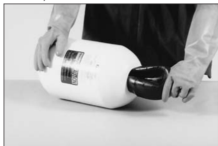
9 Remove the O-ring, O-ring back-up and metal back-up rings ( avoid letting these items fall into the shell; it will be difficult to retrieve these items, especially if your accumulators are vertically mounted ).
