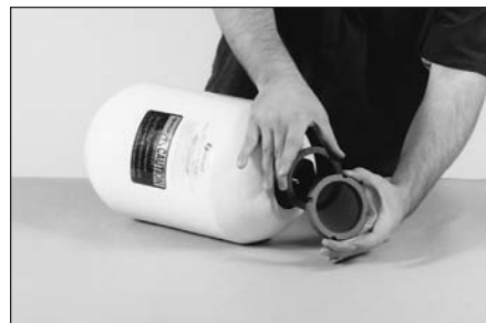
4 Once the remaining nitrogen has been discharged, remove the valve adapter using a socket wrench. (*If accumulator is mounted vertically, perform steps 5 through 12 before performing this step).
