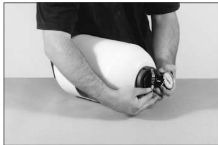
3 Discharge any pressure in the accumulator using the OilAir Hydraulics charging and gauging assembly, OAH Part number TCG-3000 (or CG-5000 for 5 kpsi models).
