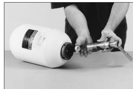
7 Install the OilAir Charging & Gauging assembly on to the valve adapter and fill the accumulator with Nitrogen up to 30 psig (2 bar). This helps to seat the port adapter and anti-extrusion ring into the shell opening. Remove the C & G assembly.
