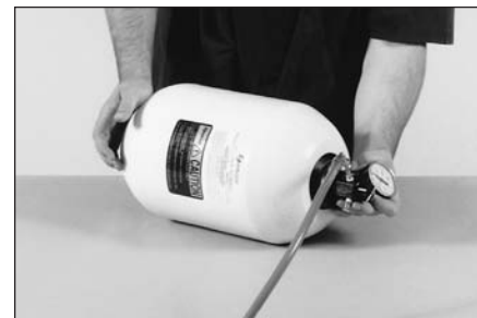
4 Insert the port adapter carefully into the shell. Be careful not to drop the port adapter into the shell! Slide the valve stem of the bladder through the port adapter.
