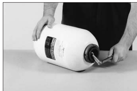
1 Removal from the system After removing all hydraulic pressure from the system, remove the protective cap from the valve stem.
