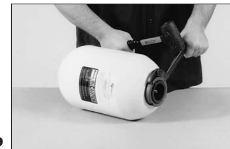
6 Carefully pull the port adapter through the anti extrusion ring and on through the port opening of the shell.
