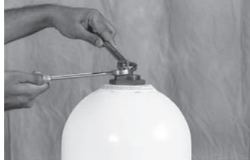
2. Open the valve adapter by securing the bottom hex with a wrench while turning the top hex counter clockwise.
