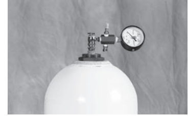
4. Install Charging and Gauging Assembly on the accumulator by screwing the air chuck to the gas valve. Hand tighten sufficiently to prevent any leakage. Connect the hose to the nitrogen bottle regulator.
