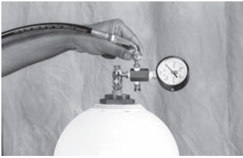
5. Remove the seal cap from the gas charging tank valve and connect the swivel connector on the hose assembly. Hand tighten sufficiently to prevent leakage.
