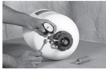
3. Close the bleed valve on the charging and gauging assembly.
