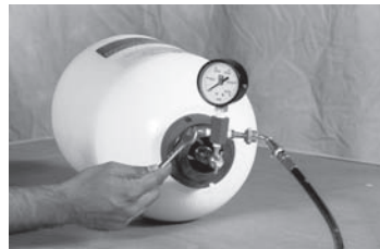
8. Open the bleed valve to bleed of nitrogen in the hose. Disconnect the charging assembly from the accumulator and the gas bottle.
