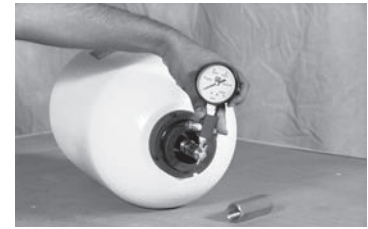
4. Install Charging and Gauging Assembly on the accumulator by screwing the air chuck to the gas valve. Hand tighten sufficiently to prevent any leakage. Connect the hose to the nitrogen bottle regulator.
